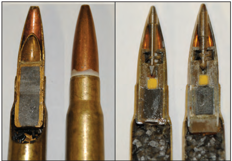
Above: The construction of some bullets can be quite complex. At the left is a Japanese 7.9 x 57 explosive round and at the right are German explosive bullets by Polte, Magdeburg revealing the complex striker mechanism.
