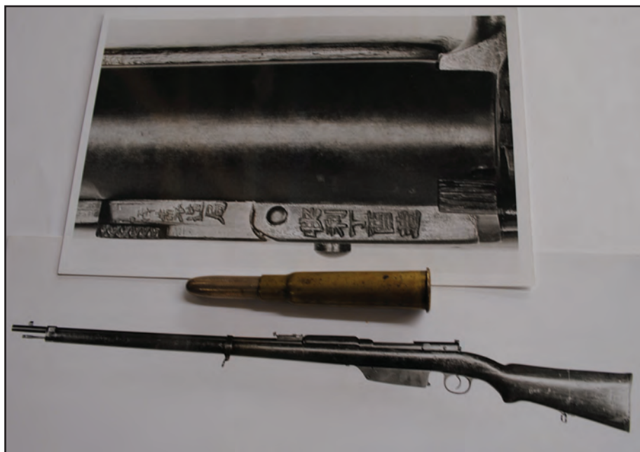
Above: The cartridge in search of a rifle. Through his colleague, Herbert Woodend, at the British Ministry of Defense Pattern Room, Bill Woodin was able to match this rare cartridge he named the “7.62x55R” with an equally rare Chinese version of the 8mm Austrian Model 1888-90 Mannlicher (pictures with closeup of receiver markings.) This type of detective work is what Bill describes as the “thrill of discovery.” But some of the ongoing work involves real-world police and military investigations.
