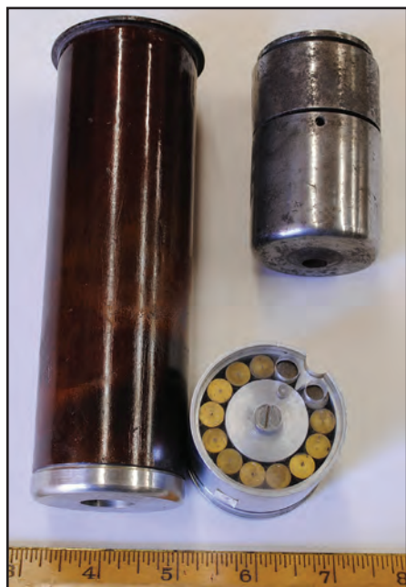
Above: Cartridge design by the Hungarian Bela Zettl during WW2. Upper right: original 7.9mm prototype (only known specimen). Others are later U.S. experiments with this design in .30 cal. These had an extremely high rate of fire - up to 45,000 rpm - but a satisfactory feed system and weapon were never developed.
