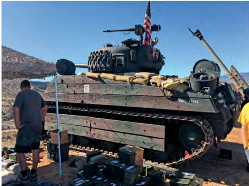
Big Sandy shoot (2019). Sherman Tank modified as a "Ronson" or "Zippo" flamethrower on Iwo Jima. The sides were protected from magnetic mines by wooden planks attached to the sides. Restored by Battleground Las Vegas.
