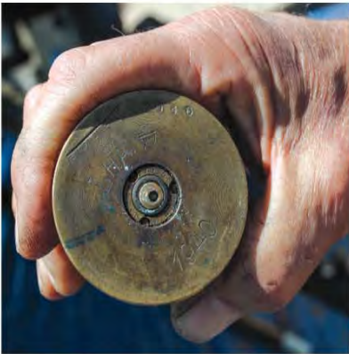
Old rounds nearly a century old can have corroded primers or be unstable and dangerous. At the J. Curtis Earl shoot, the Bofors ammunition would not fire due to primer failure. Luckily, it did not explode.
