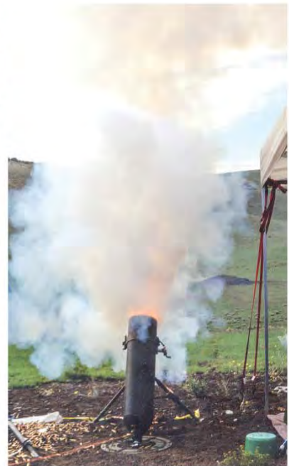
Gas cylinder bowling ball mortars are real crowd-pleasers. The ball goes up a quarter mile and "pulse whistles" on the way down as air blows past the rotating finger holes.
