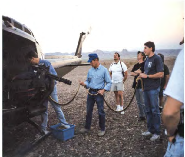
A belt of solid tracers is fed into the 4,000-round ammo container.
