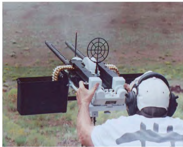
SP Crater 2003. Twin AN-M2 30 cal. Brownings. These were owned by Mike Dillon and came from the rear of a Douglas SBD Dauntless dive bomber. Combined, the pair have a rate of fire like a Minigun. (Kenton Tucker)
