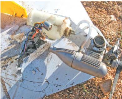
RC model target plane designs have evolved so that only a direct hit to a vital part brings them down. This 4th generation one took hits to both its engine and receiver.
