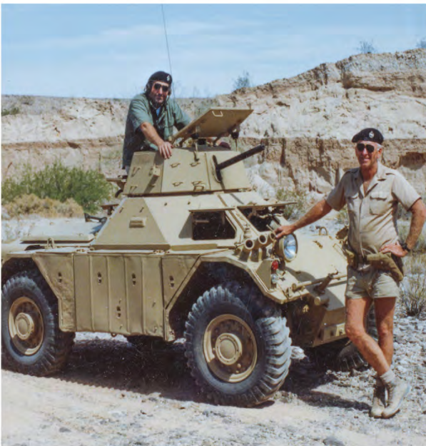
Bob Faris in Yuma looking rather dapper in front of a Mark 2 Ferret with a 30 cal. Browning in a traversable turret. Faris claimed that the US Border Patrol was astonished to see it. No doubt. (Kenton Tucker)
