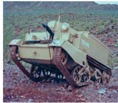
British Bren Gun Carrier Mk II (a.k.a. Universal Carrier) cresting a hill at a Marana Shoot. One of the more unusual armored vehicles; this one armed with a Vickers. (Ed Hope)
