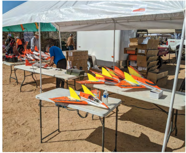
The latest evolution in airplane targets. These are 6th generation "pusher electric" RC models that travel over 100MPH. (Ron Lippert)
