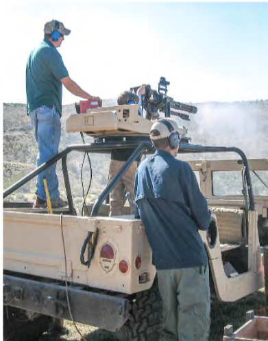
Hummer mounted Dillon Aero Mini gun. At 2,000-6,000 RPM, it will fill up the Hummer truck bed fast.
