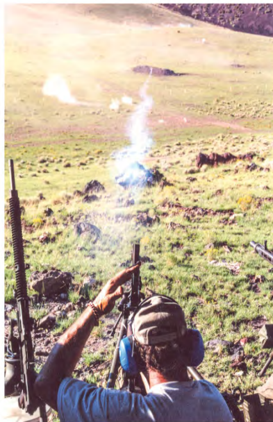
Rare British .303 smoke tracer fired from a Bren. The bullet leaves a spiraling smoke trail from phosphorus spun out of a weep hole and igniting on contact with the air. SP Crater Shoot circa 1998.
