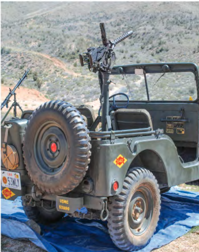
New Vs. Old: 600RPM 1919 A4 Browning mounted on an M38A1 Willys Jeep with a 1917 Browning cradle.
