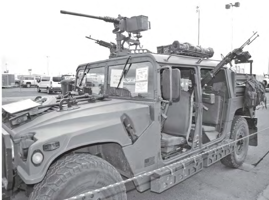
The Arizona Military Vehicle Collectors Club displayed a collection of meticulously restored vehicles from WWII forward in front of the SAR West building. Impractical but fascinating to view, this Humvee bristled with (front to back) an M2HB 50, an M60, an inert AT4 Anti-Tank Weapon, an M240, and a III Модернизированный (a.k.a, Russian PKM).
